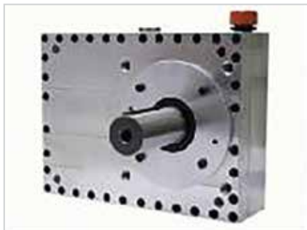
S3143 speed and torque first will be angled by 105 degree via bevel gear and direction of rotation inverted, 1:1 ratio. After that spur gears invert the direction of rotation again ratio 1.05
