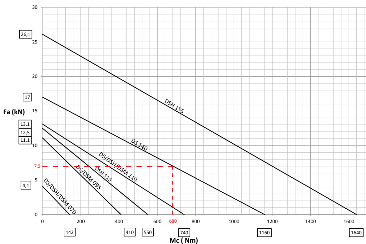
Fig. 9.2: Allowable load for the tilting moment and the axial force
