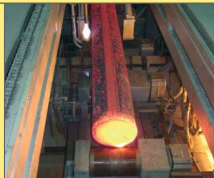
Roller conveyor drive with water-cooled angle parallel shaft geared motors
